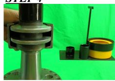
Choose the clamshell that best fits your bearing / race. After choosing, place one half over puller as shown and adjust top ring to ensure there is no vertical play inside clamshell. Once that is accomplished, position second 1/2 of clamshell around rings.
